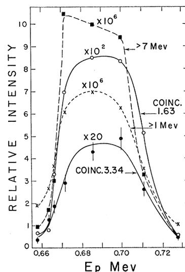
FIG. 4. Yield curves measured at the 669-keV resonance in the proton bombardment of  $\text{F}^{19}$ . They are, respectively, the yield of all gamma rays of energy greater than 1 MeV (crosses), of all gamma rays of energy greater than 7 MeV (squares), of 1.63-MeV gamma rays in coincidence with 11.88-MeV gamma rays (open circles), and of 3.34-MeV gamma rays in coincidence with primaries feeding the 4.97-MeV level in  $\text{Ne}^{20}$  (closed circles).
