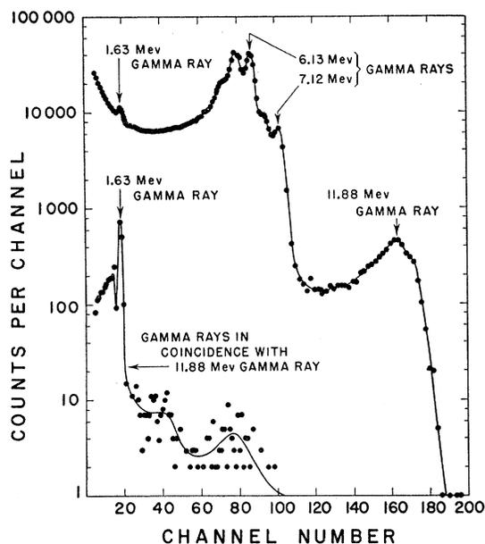
FIG. 2. The upper curve shows the direct gamma-ray pulse spectrum measured at the 669-keV resonance in the proton bombardment of  $\text{F}^{19}$ . The lower curve is the spectrum in coincidence with pulses corresponding to 11.88-MeV gamma rays.
