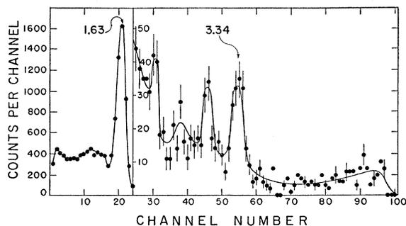
FIG. 3. The pulse spectrum at the 669-keV resonance corresponding to gamma rays in coincidence with gamma rays of energy greater than 7 MeV measured in a second detector.
