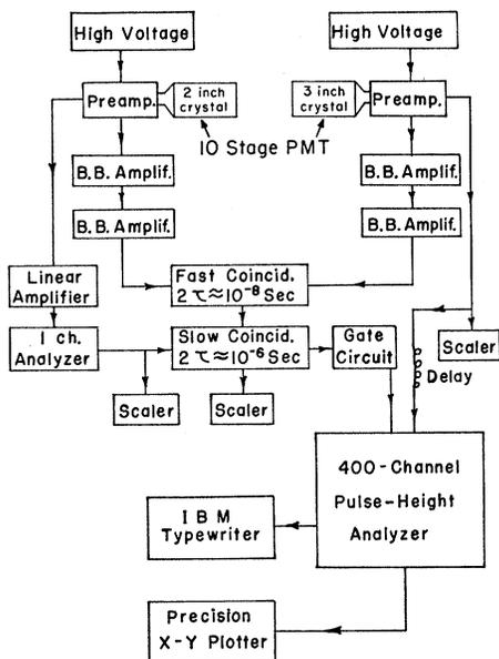
FIG. 1. Coincidence spectrometer.
