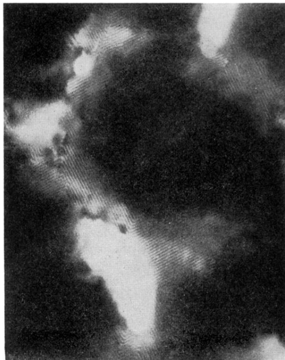
FIG. 5. Electron micrograph of CuAu II showing antiphase domain structure. Magnification 320 000 \times .
