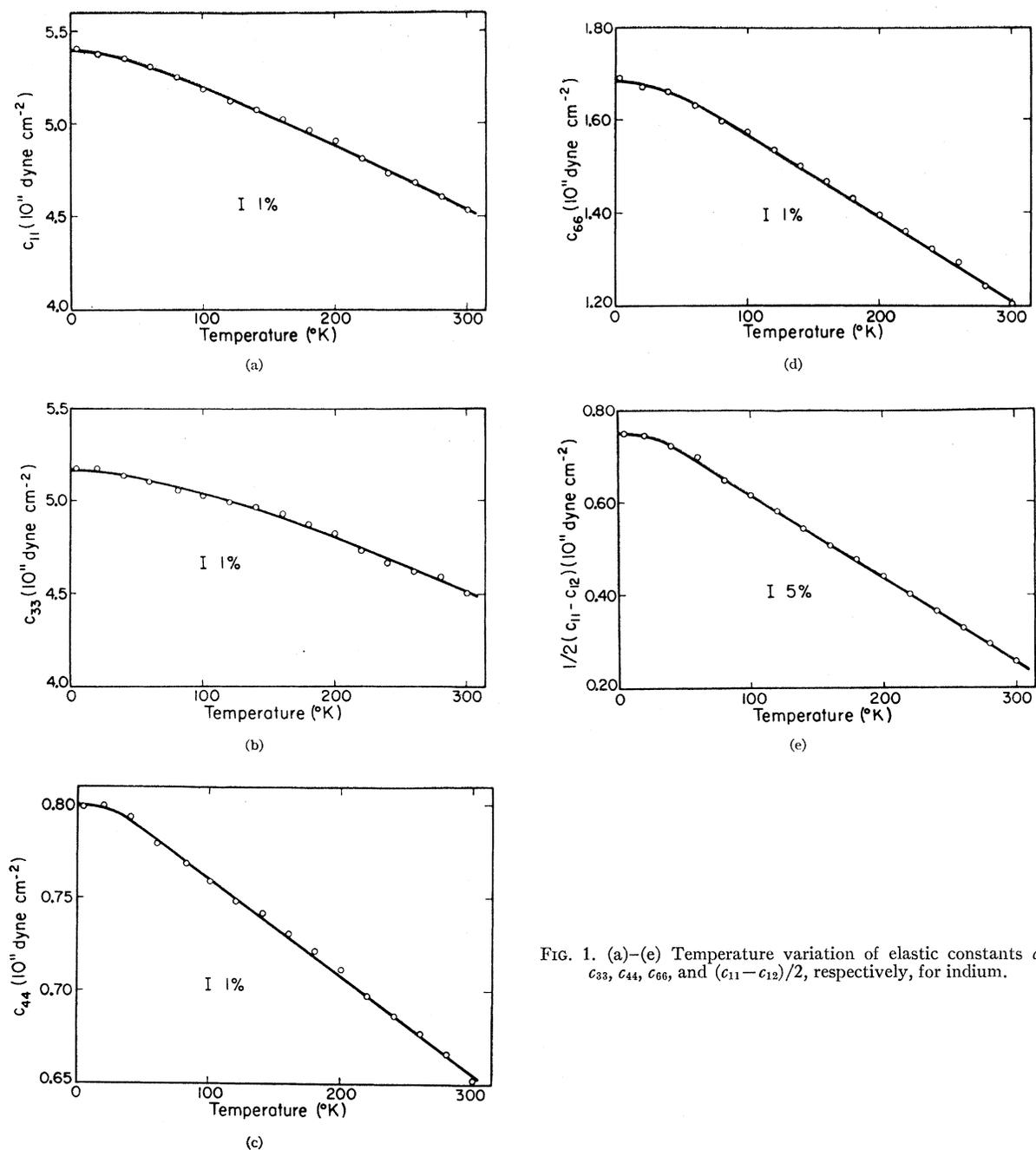
FIG. 1. (a)–(e) Temperature variation of elastic constants  $c_{11}$ ,  $c_{33}$ ,  $c_{44}$ ,  $c_{66}$ , and  $(c_{11} - c_{12})/2$ , respectively, for indium.
