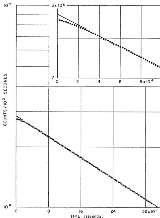
Fig. 6. Decay curve for  $Y^{90}$  ground-state beta activity.
