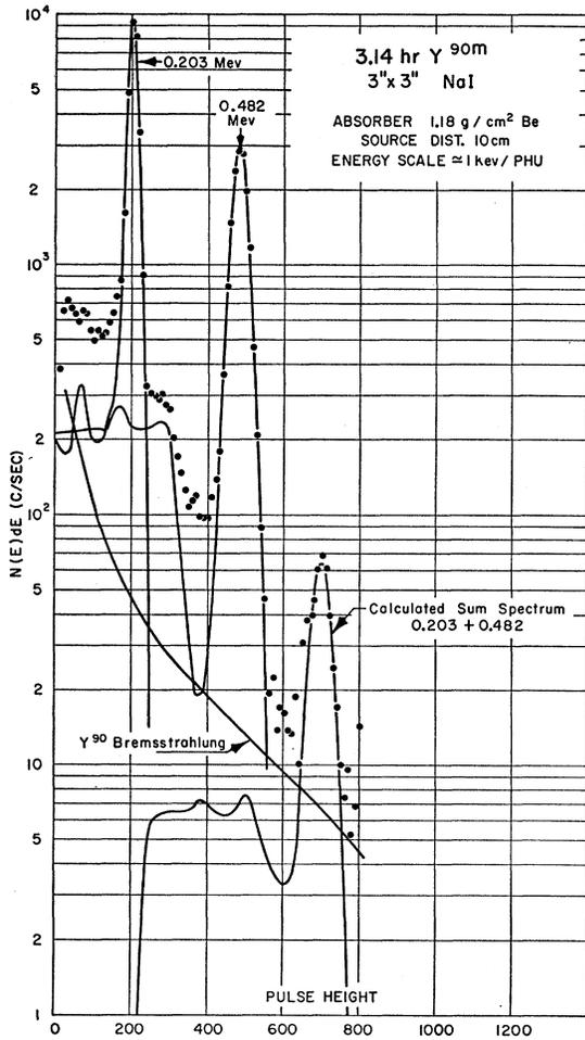
FIG. 1. Gamma-ray spectrum of 3.14-hr  $Y^{90}$  showing sum spectrum.
