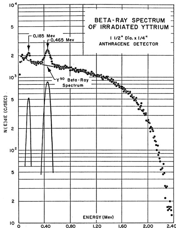
FIG. 4. Spectrum of beta radiation from yttrium sample.
