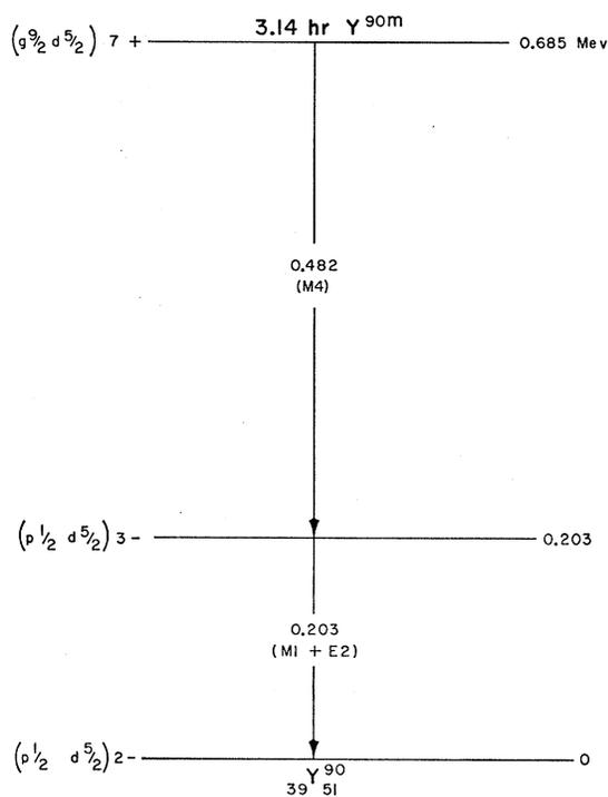
FIG. 8. Level scheme for  $Y^{90m}$ .
