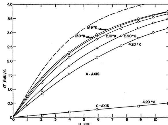
Fig. 6. Magnetization  $\sigma$  in emu/g vs magnetic-field strength  $H$  in koe for the 1.0 at. % Ho single crystal. The lowest curve is for  $H$  parallel to the  $c$  axis, whereas the upper curves are for  $H$  parallel to the  $a$  axis. The dashed curve represents the expected behavior of an ideal paramagnetic material of saturation moment 4.8 emu/g at 1.49°K.
