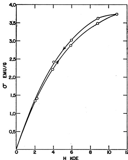
Fig. 7.  $\sigma$  versus  $H$  at 1.58°K for the 1.0 at. % Ho single crystal with field increasing and decreasing and with the  $a$  axis parallel to the field.
