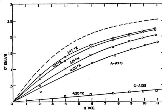
Fig. 5. Magnetization  $\sigma$  in emu/g vs magnetic-field strength  $H$  in koe for the 0.6 at. % Ho single crystal. The lowest curve is for  $H$  parallel to the  $c$  axis, whereas the upper curves are for  $H$  parallel to the  $a$  axis. The dashed curve represents the expected behavior of an ideal paramagnetic material of saturation moment 2.9 emu/g at 1.47°K.
