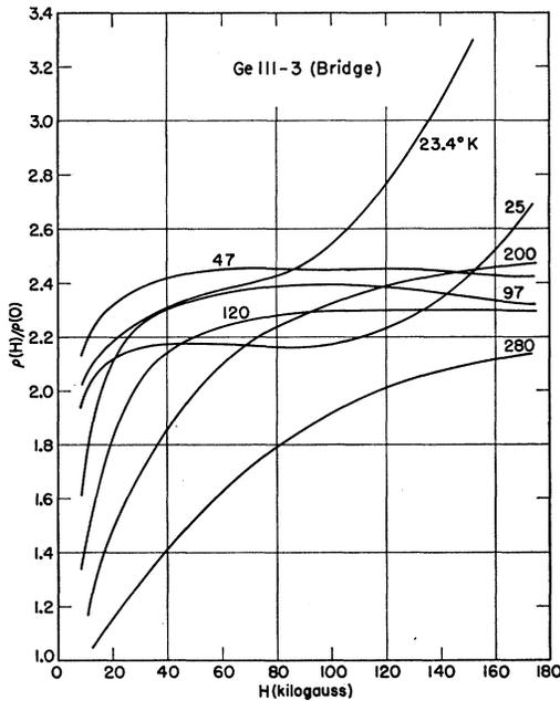
FIG. 4. Curves of  $\rho(H)/\rho(0)$  vs  $H$  with temperature as a parameter for Ge 111-3.
