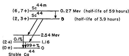
FIG. 1. Decay schemes of  $\text{Sc}^{44m}$  and  $\text{Sc}^{44}$ .
