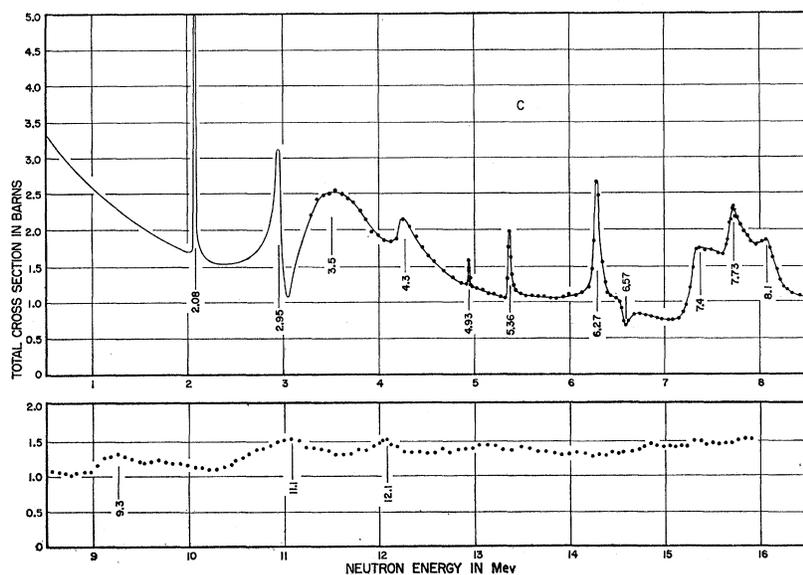
FIG. 4. The total cross section of C. The curve up to 3.4 Mev represents measurements from references 6 and 7. Except at the sharp peaks where all the measurements are shown, each dot is an average of three data points below 7 Mev and of two data points above this energy. Statistical errors are less than 3%. The neutron energy spread is about 20 kev up to 7 Mev and above this energy about 45 kev.
