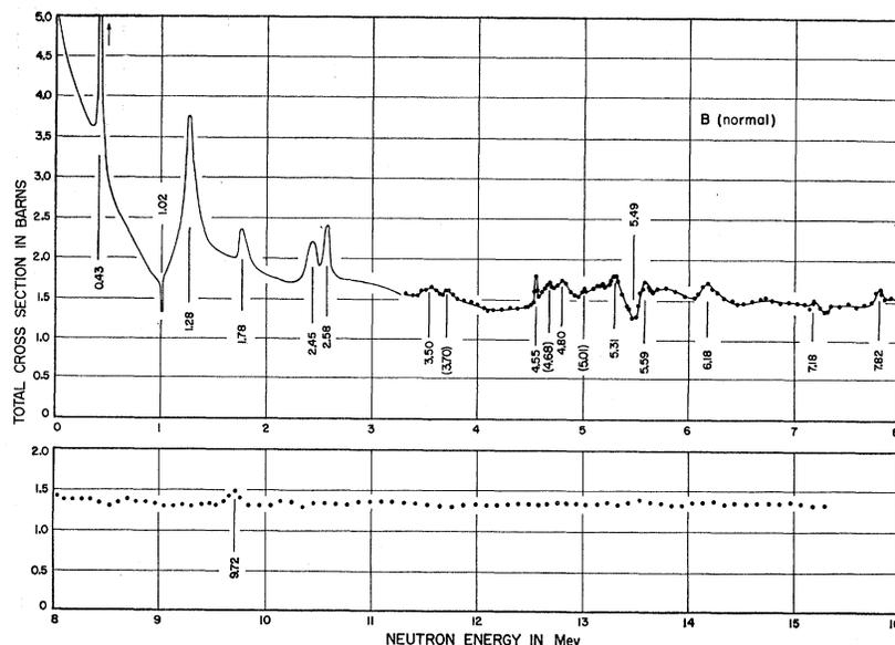
FIG. 3. The total cross section of normal B. The curve up to 3.4 Mev represents measurements from references 6, 7, and 12. Except at the sharp peaks where all the measurements are shown, each dot is an average of two data points. Statistical errors are less than 3%. The neutron energy spread is about 30 kev up to 9.5 Mev and above this energy about 45 kev.
