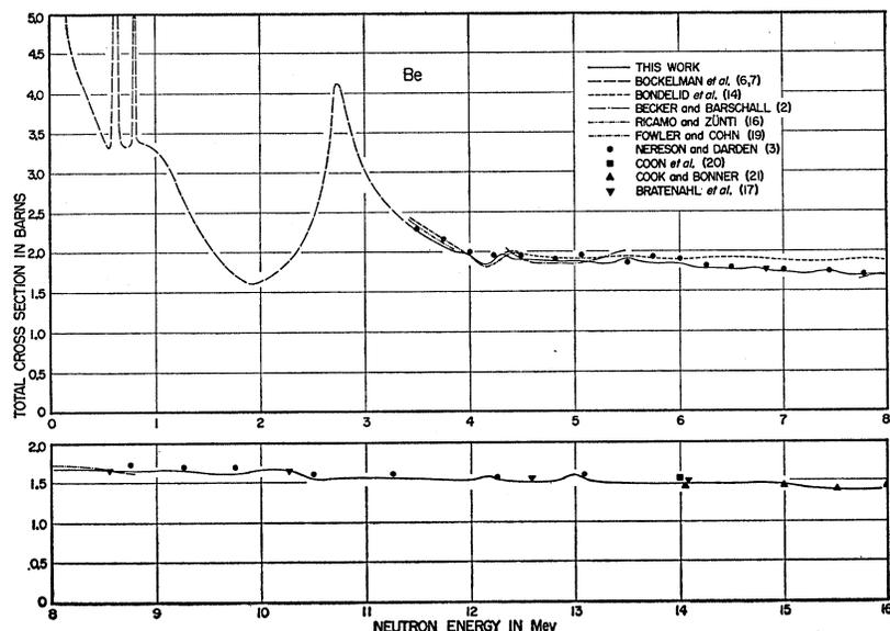
FIG. 7. The total neutron cross section of Be is compared with previous measurements from the indicated references.
