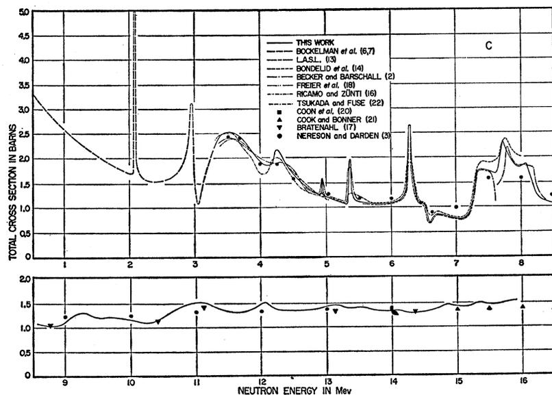
FIG. 8. The total cross section of C is compared with previous measurements from the indicated references.
