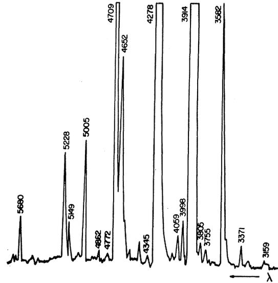
Fig. 3. Spectrogram of 200-keV proton impact on  $N_2$  (17  $\mu$  pressure and 0.14  $\mu$ a beam current).
