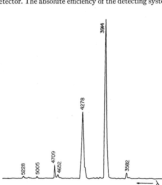
FIG. 1. Spectrogram of 200-keV proton impact on  $N_2$  (19- $\mu$  pressure and 0.04- $\mu$  beam current).
