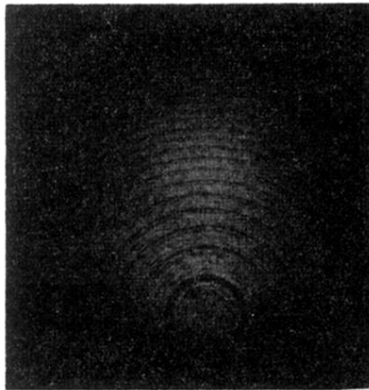
FIG. 16. Stimulated emission from ruby as observed through a Fabry-Perot interferometer having an 18.5-cm plate separation (interorder spacing 0.0135 Å). Bright fringes are the white areas of the figure.
