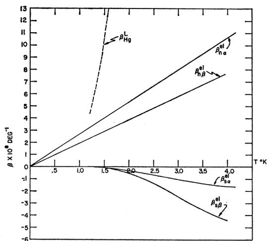
FIG. 4. Comparison of the various contributions to the thermal expansion of  $\alpha$ - and  $\beta$ -Hg. The lattice contribution was calculated from experimental specific heat data using an estimated Grüneisen constant of 2.
