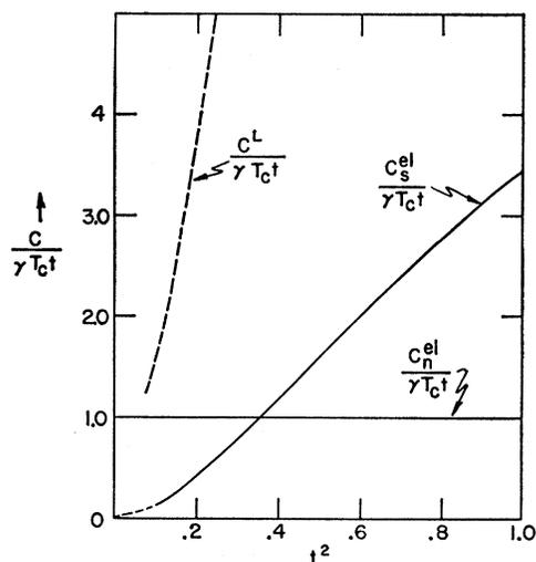
FIG. 3. Contributions to the specific heats of  $\alpha$ - and  $\beta$ -Hg. The electronic contributions are identical for the two phases on this plot which is expressed in reduced variables. The lattice contribution is given by Smith and Wolcott (reference 3).
