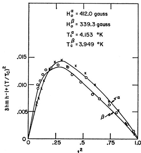
FIG. 1. A plot of the deviation from parabolic behavior of the critical field curves for  $\alpha$ - and  $\beta$ -Hg. The solid curves are the results of least-squares power series fits to all the experimental data, while the points shown represent typical runs. The maximum difference between the two curves corresponds to, roughly, 0.4 gauss.
