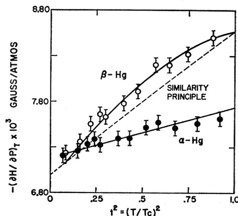
FIG. 2.  $(\partial H_c / \partial P)_T$  for  $\alpha$ - and  $\beta$ -Hg. The solid curves are the results of least-squares power-series fits to the experimental data while the points shown represent typical runs. Each run was made at a fixed pressure, the magnitude of which was uncertain to 3%.
