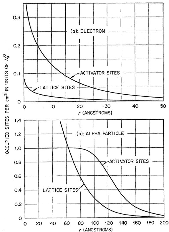
FIG. 9. Distribution of energy carriers on activator sites and trapping sites after the diffusion and capture processes are complete. (a) Low- $dE/dx$  case corresponding to incident electron of 0.15 Mev. (b) High- $dE/dx$  case corresponding to 4-Mev alpha. Note different scales in (a) and (b). Curves apply to NaI(Tl) of activator concentration  $\sim 1 \times 10^{-3}$ .
