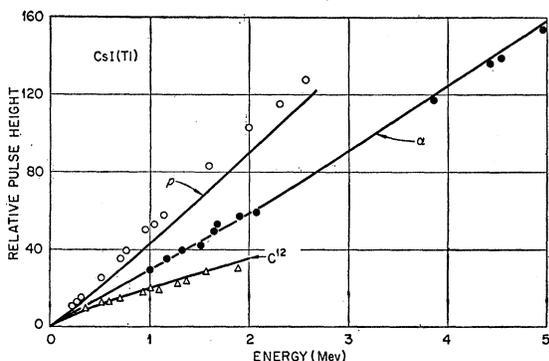
FIG. 7. Calculated pulse height versus energy for  $p$ ,  $\alpha$ , and  $C^{12}$  in CsI(Tl), superimposed on experimental data from reference 22. Calculated curves are based on smooth curve of Fig. 6 and are normalized to experimental points for alphas between 1 and 2 Mev.
