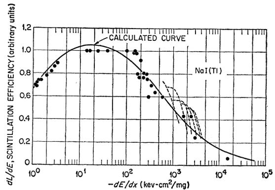
FIG. 6. Calculated scintillation efficiency versus  $dE/dx$  superimposed on experimental data. The normalization and choice of  $\alpha K = 2(\text{kev-cm}^2/\text{mg})^{-1}$  are chosen to give a best fit with experiment.
