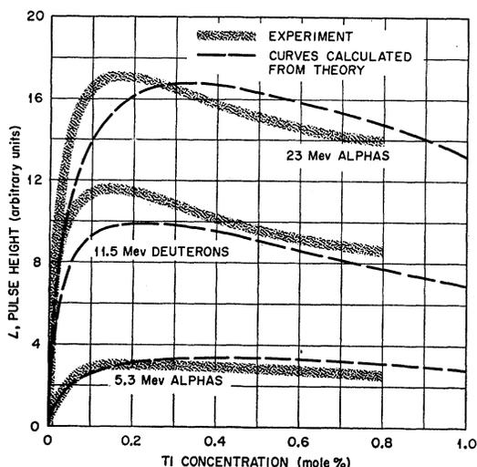
FIG. 11. Pulse height versus Tl concentration for different particles on NaI(Tl). Experimental curves from Eby and Jentschke, reference 8. Calculated curves result from integration of curves in Fig. 10, and are normalized to experiment with the choice of one constant.
