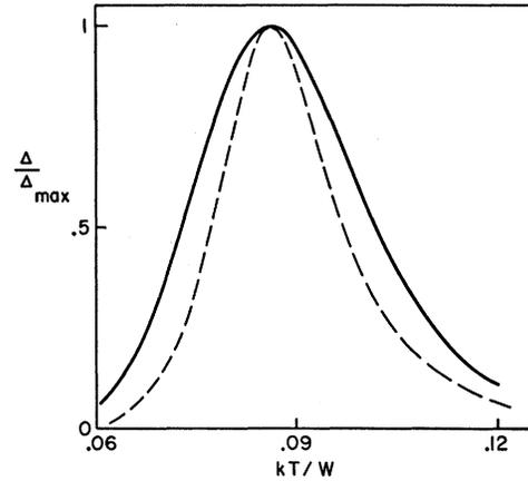
FIG. 2. The internal friction as a function of temperature. The full curve was calculated from the theory, for a value of the frequency given by  $(\omega l^2/D_0\pi^2) = 10^{-6}$ . The broken curve corresponds to a single relaxation process with the same peak temperature.
