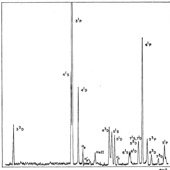
FIG. 4. Spectrogram reproduction from 200-keV proton impact on helium at 26- $\mu$  pressure and with a beam current of 0.18  $\mu$ a. Helium lines are labeled by the upper state.  $H_{\beta}'$  represents the Doppler-shifted  $H_{\beta}$  line.
