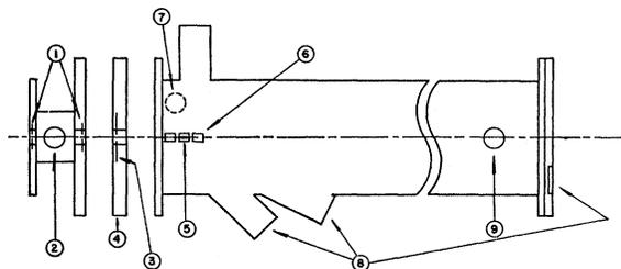
FIG. 1. Details of collision chamber. (1) beam collimating holes ( $\frac{1}{16}$  in.), (2) differential pumping outlet, (3) electron repeller, (4) Lucite spacer, (5) observation region, (6) plates to apply an electric field across the observation region, (7) Pirani gauge, (8) observation ports, (9) target gas inlet.
