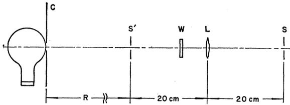
FIG. 3. Calibration of spectrometer. The standard lamp with associated diaphragm  $C$  is placed a distance  $R$  from the entrance window  $S'$  (image of the spectrometer entrance slit  $S$  formed by the fused-quartz lens  $L$ ).  $W$  is the fused-quartz window used on the collision chamber.
