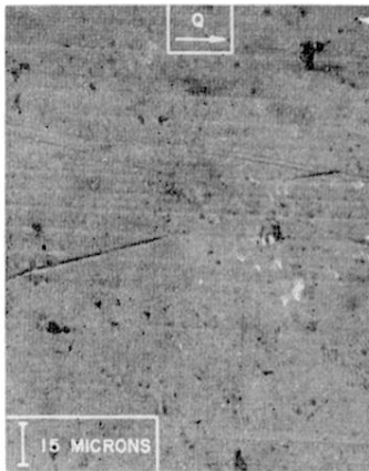
FIG. 7. Bright-field photomicrograph of etched surface of Ge+0.77 at. % Si sample. The interval indicated on the photograph is equivalent to 15 microns on specimen. Arrow indicates direction of heat flow during thermal conductivity measurements.
