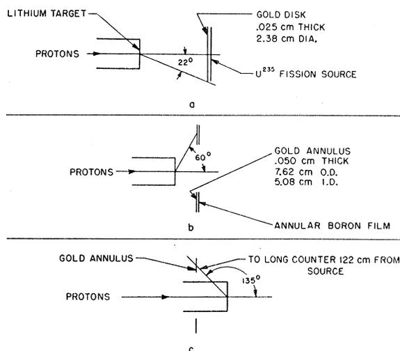
FIG. 1. The experimental arrangement for activation measurements from  $E_n = 200$  keV to  $E_n = 1500$  keV is shown in Fig. 1(a). Fig. 1(b) and 1(c) show the experimental arrangements for activation measurements from  $E_n = 30$  keV to  $E_n = 200$  keV.
