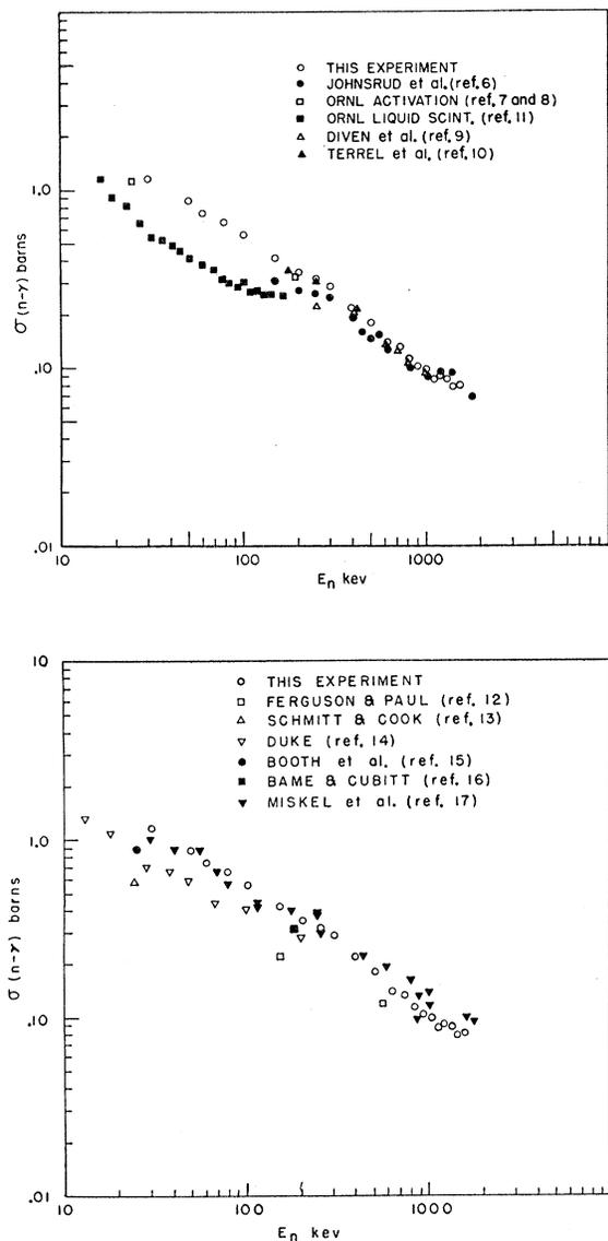
FIG. 2. Comparison of gold neutron capture cross-section measurements.
