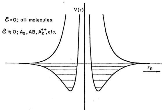
Fig. 2. The nuclear potential for a diatomic molecular system in the absence of an electric field. The vibrational states are indicated schematically by the light horizontal lines. In the presence of an electric field this potential remains unperturbed in lowest order for heteronuclear molecules and homonuclear systems in even charge states.
