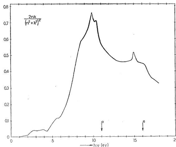
FIG. 4. Imaginary part of the reciprocal of the complex dielectric constant for Ge as calculated from dispersion relations. Vertical lines marked  $e$  denote positions of observed energy characteristic losses.
