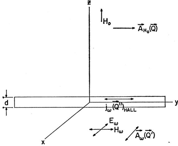
FIG. 4. Geometry for transverse Hall current in superconductor.
