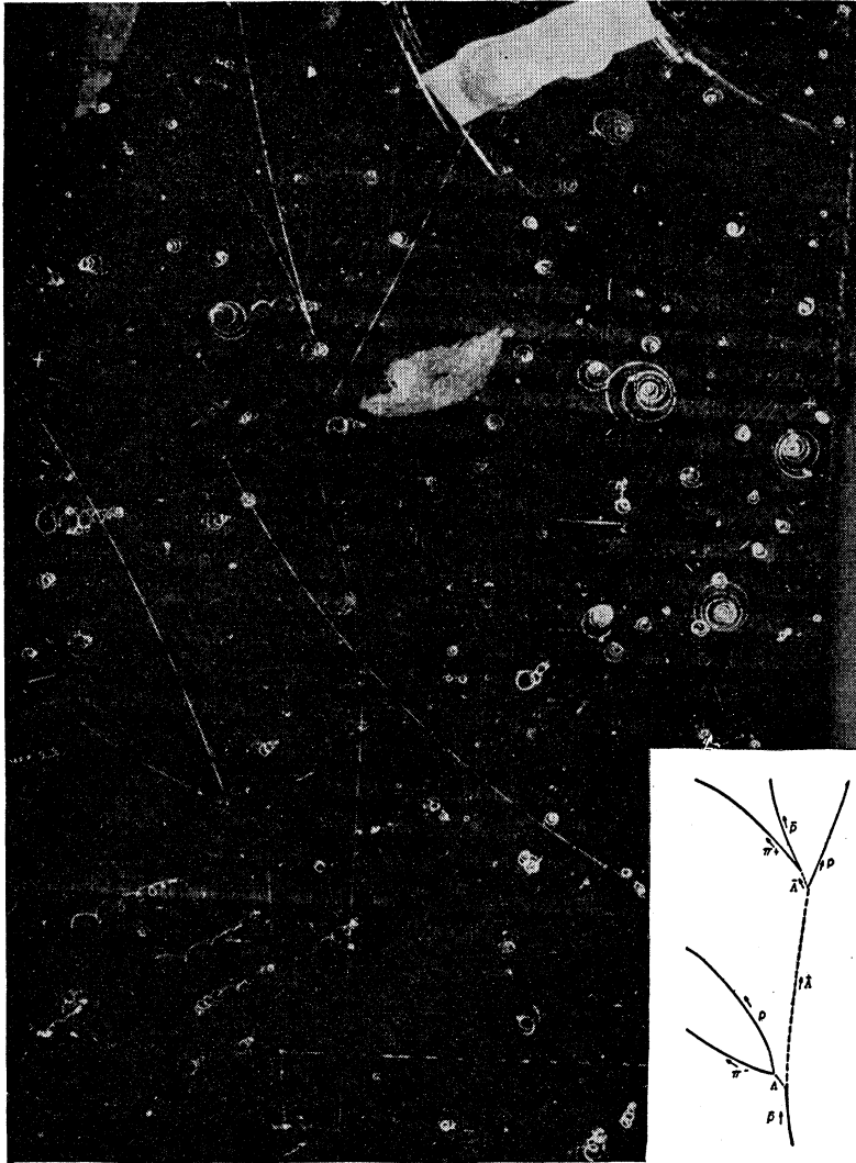
FIG. 11. Production of anti-lambda and lambda hyperons by antiproton annihilation. The anti-lambda scatters from a target proton.
