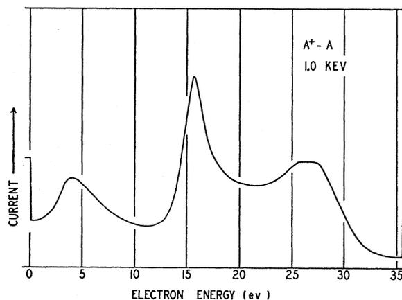
FIG. 2. Sample data record for 1.0-kev  $\text{A}^+$  in A. The analyzer deflection voltage increases from left to right. The small peak on the left represents secondary electrons from the cylinder walls.
