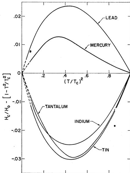
FIG. 3. Deviation of critical field curves of several superconductors from parabolicity. For clarity the curves for individual samples of tin and indium are not shown (since the differences in  $D$  amount to 0.0014 or less).
