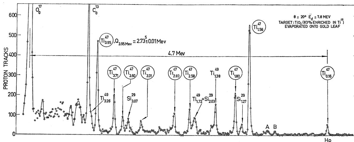
FIG. 2. The  $20^\circ$   $(d,p)$  spectrum from a  $TiO_2$  target enriched to 83% in  $Ti^{46}$ . The augmentation of peaks corresponding to  $Ti^{46}$  and the diminution of those corresponding to  $Ti^{48}$ , as compared with Fig. 1, is commensurate with the isotopic composition of the targets. Such comparison, together with the examination of the kinematic behavior, led to the identification of four new levels in  $Ti^{47}$ .
