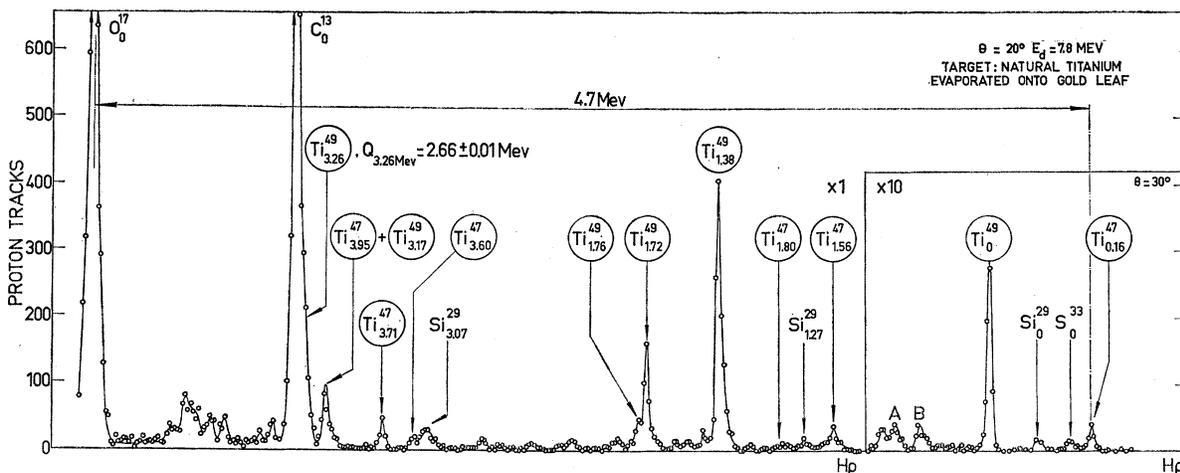
FIG. 1. The  $(d,p)$  spectrum from a natural titanium target. This spectrum is a composite of six overlapping partial spectra registered in nuclear emulsions at the image plane of a high resolution magnetic spectrometer. Except for the high-energy portion, for which the  $Ti^{49}$  and  $Ti^{47} l_n = 3$  transitions are stronger at  $30^\circ$ , the spectrum is composed from  $20^\circ$  data. All peaks are labeled by the residual nucleus.
