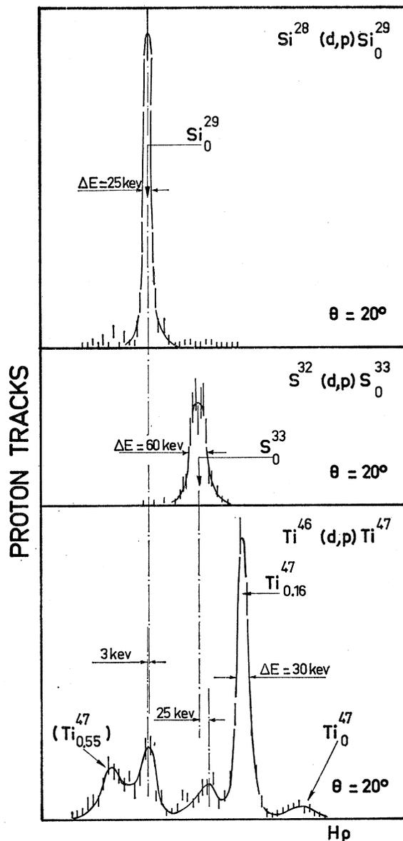
FIG. 4. Comparison of spectra taken under identical conditions off S, Si, and  $Ti^{46}O_2$  targets. This juxtaposition served as a double check in the identification of the ground state and the 0.55-Mev state in  $Ti^{47}$ ; it helped in making a positive identification of the  $S^{29}$  and  $S^{32}$  impurity groups in the  $Ti^{46}(d,p)Ti^{47}$  spectrum.
