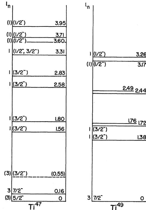
FIG. 9. Energy level diagrams for Ti<sup>47</sup> and Ti<sup>49</sup>. Levels at (0.55), 1.80, 3.60, and 3.71 Mev in Ti<sup>47</sup> and at 2.44 Mev in Ti<sup>49</sup> have not been reported previously. Known spins, and those assigned in Sec. IV of this paper, are shown next to the corresponding levels.
