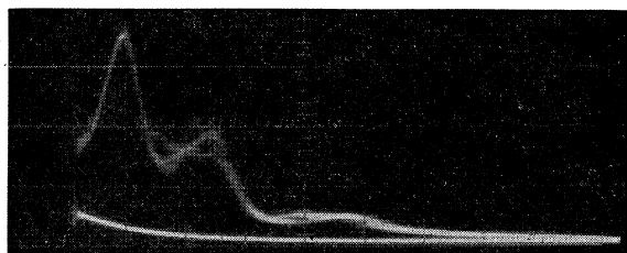
FIG. 5. Switching current transient of sodium vanadate-niobate \text{Na}(\text{V}_{0.2}\text{Nb}_{0.8})\text{O}_3 at room temperature, with an applied potential of 125 volts and 250 volts; switching time \tau_s = 6 \mu sec and maximum switching current i_{\text{max}} = 0.4 ma.
