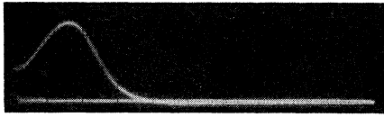
FIG. 7. Switching current transient of sodium-silver niobate (\text{Na}_{0.9}\text{Ag}_{0.1})\text{NbO}_3 with an applied potential of 125 volts and 250 volts; switching time \tau_s = 15 \mu\text{sec} and maximum switching current i_{\text{max}} = 4.8 \text{ ma} .
