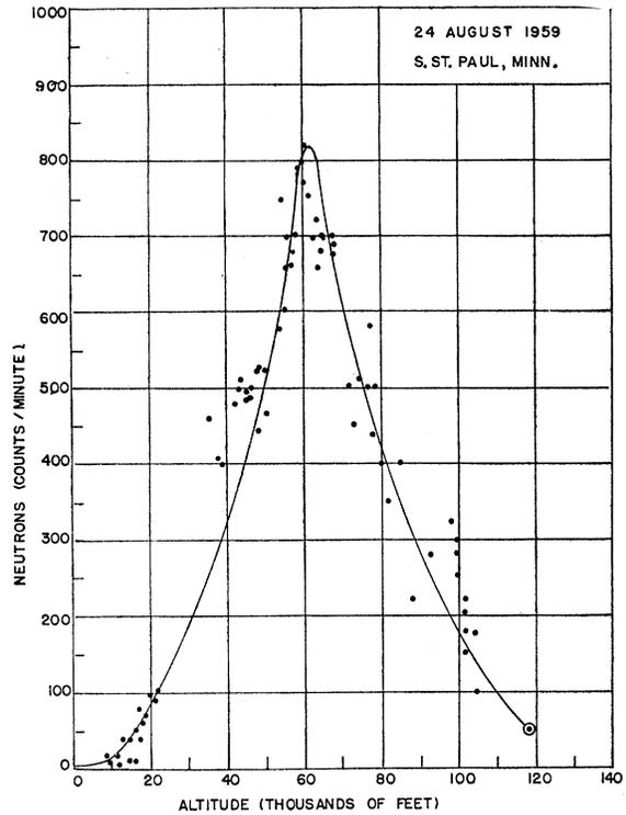
FIG. 3. Slow-neutron density as a function of altitude. The high altitude point represents three hours at ceiling.
