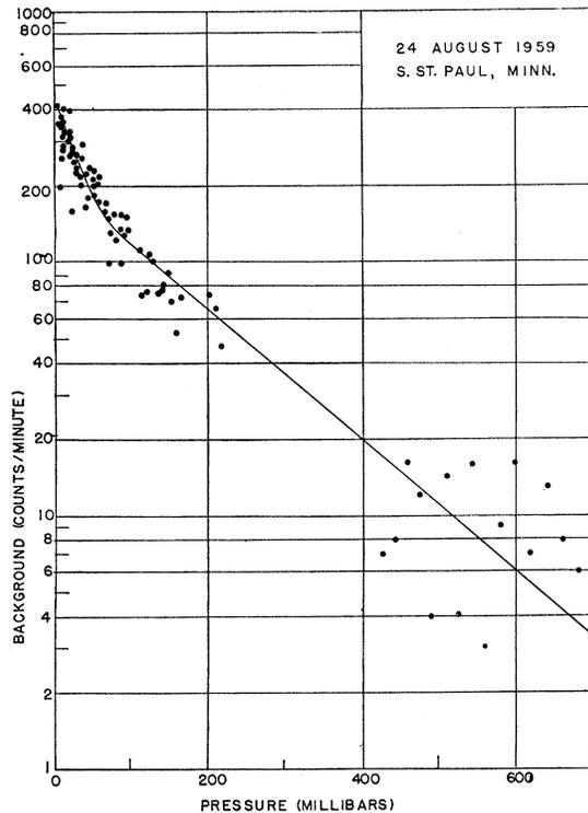
FIG. 4. Background radiation as a function of atmospheric pressure. This system detects those events which liberate more than 2 Mev in the counter.
