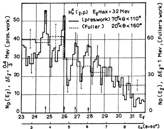
FIG. 3. Photoproton spectrum from He in  $\Delta E_\gamma$  steps of 0.133 Mev;  $70^\circ < \theta < 110^\circ$  (plates parallel to the  $\gamma$  beam). The correspondence between  $E_p$  and  $E_\gamma$  for  $\theta=90^\circ$  is reported. The statistical [root mean square errors are indicated. The legend on the left-hand side of the figure should read 0.133, rather than 0.4/3.
