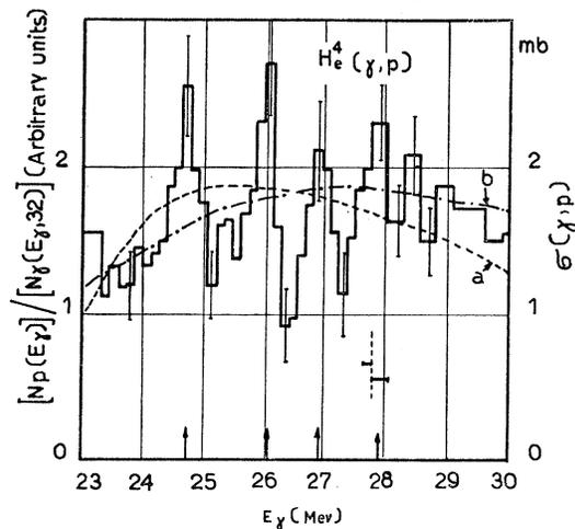
FIG. 4. Histogram: He( $\gamma, p$ ) differential cross section derived from the  $90^\circ \pm 20^\circ$  spectrum of Fig. 3 (present work) in arbitrary units. Curve (a): He( $\gamma, p$ ) cross section in millibarns according to Fuller.<sup>2</sup> Curve (b): He( $\gamma, p$ ) cross section in millibarns according to Gorbunov and Spiridonov.<sup>3</sup>
