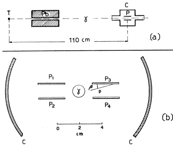
FIG. 1. (a) Experimental arrangement; (b) disposition of the photoplates.  $T$ =target of the betatron;  $Pb$ =lead collimator;  $C$ =chamber filled with He;  $P$ =nuclear photoplates 1 in.  $\times$  3 in. parallel to the  $\gamma$  beam;  $\gamma$ =collimated  $\gamma$ -ray beam from the betatron;  $p$ =photoproton.
