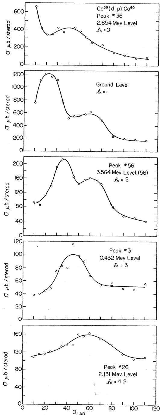
FIG. 2. Examples of experimental angular distributions of protons with the  $l_n$  value of the captured neutrons as indicated on each individual graph. The curves are smooth experimental curves, not theoretical ones.
