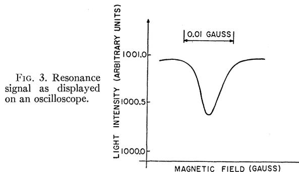
FIG. 3. Resonance signal as displayed on an oscilloscope.
