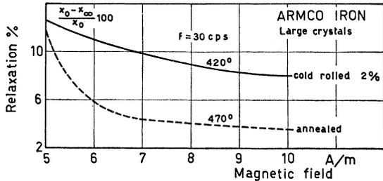
FIG. 1. Relative change of susceptibility (in percent) vs magnetic field, at various temperatures, of an Armco iron specimen. Broken lines: annealed; solid lines: cold rolled 2%.  $\chi_0$  taken 10 sec after demagnetization.  $\chi_\infty$  30 min later. Frequencies of the measuring field 30 cps.
