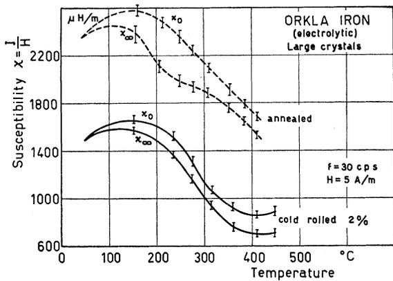
FIG. 5. Susceptibility measured 10 sec after demagnetization ( $x_0$ ) and 30 min after demagnetization ( $x_\infty$ ), of an electrolytic Orkla iron specimen. Broken lines: annealed; solid lines: cold worked 2%. Frequency of the measuring field: 30 cps. Magnetic field 5 amp-turn/m.
