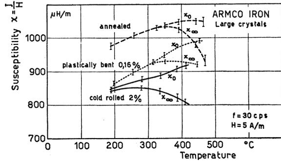
FIG. 3. Susceptibility measured 10 sec after demagnetization ( $\chi_0$ ) and 30 min after demagnetization ( $\chi_\infty$ ), of an Armco iron specimen. Broken lines: annealed; solid lines: cold rolled 2%; dotted line: plastically bent 0.16%. Frequency of the measuring field: 30 cps.
