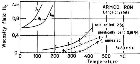
FIG. 2. Viscosity field vs temperature of an Armco iron specimen. Broken line: annealed; solid line: cold rolled 2%; dotted line: plastically bent 0.16%. Frequency of the measuring field: 30 cps.
