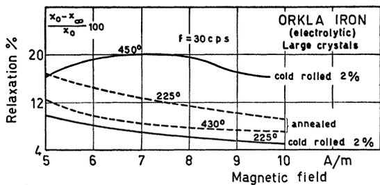
FIG. 6. Relative change of susceptibility (in percent) vs magnetic field, at various temperatures, of an Orkla iron specimen. Broken lines: annealed; solid lines: cold rolled 2%.  $x_0$  taken 10 sec. after demagnetization.  $x_\infty$  30 min later. Frequencies of the measuring field 30 cps.
