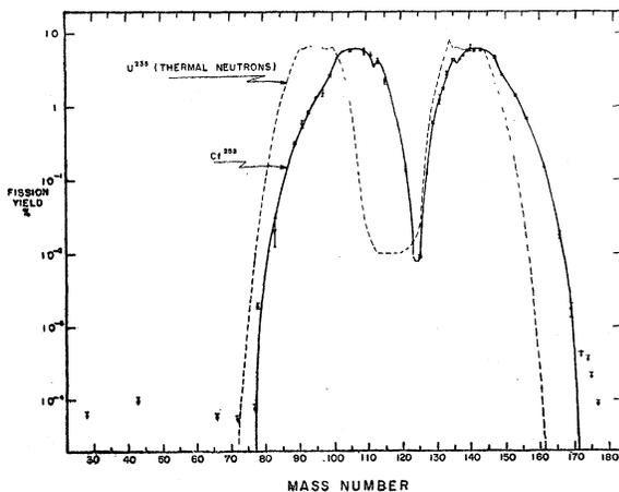
FIG. 3.  $\text{Cf}^{252}$  spontaneous fission yield as a function of mass number. All plotted points are measured, none reflected. The curve as drawn is symmetrical about mass 124.1. The yield curve for the fission of  $\text{U}^{235}$  with thermal neutrons is included for comparison.
