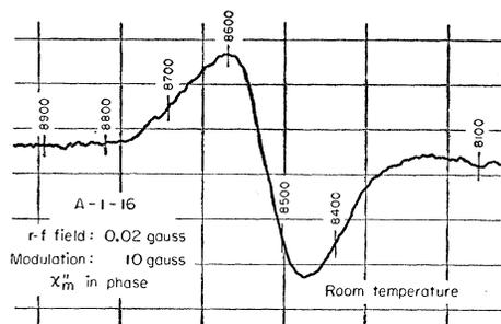
FIG. 10. Magnetic loss ( $\chi_m''$ ) in LiF.
