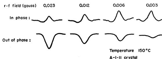
FIG. 4. The high-temperature, low-power dispersive response of LiF.
