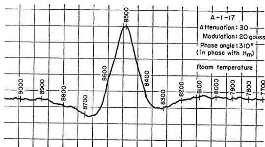
FIG. 9. The in-phase dispersion resonance in LiF.
