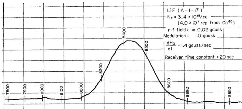
FIG. 7. The rapid-passage resonance at room temperature.
