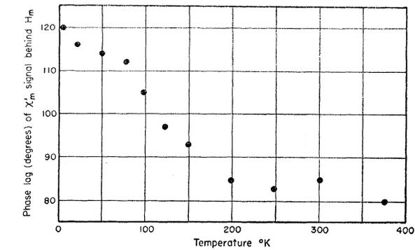
FIG. 6. Lag of rapid-passage signal  $\chi'_m$  behind modulation field as function of temperature.
