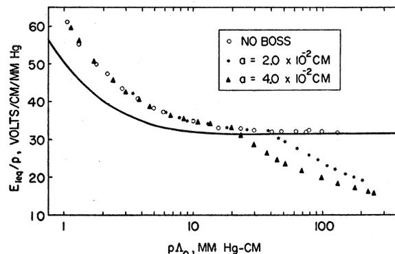
FIG. 3. Results of breakdown measurements in air at 8850 Mc/sec in the three experimental cavities.  $E_{1eq}$  is the equivalent field at the center of the cavity. The theoretical curve (solid line) would apply if breakdown were occurring in a uniform field of magnitude  $E_{1eq}$  between infinite parallel plates of separation  $L = \pi\Lambda_0$ .
