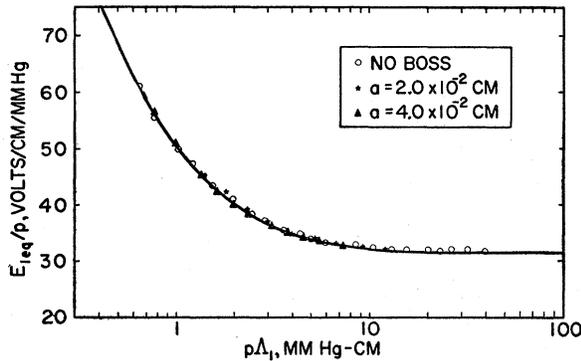
FIG. 8. Comparison of theory (solid curve) and experimental points for the region in which the boss has no effect on the cavity breakdown threshold.  $\Lambda_1 = 1/k_1$  for each experimental point was obtained from Fig. 5.
