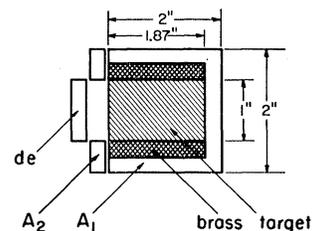
FIG. 3. Target and anticounters.
