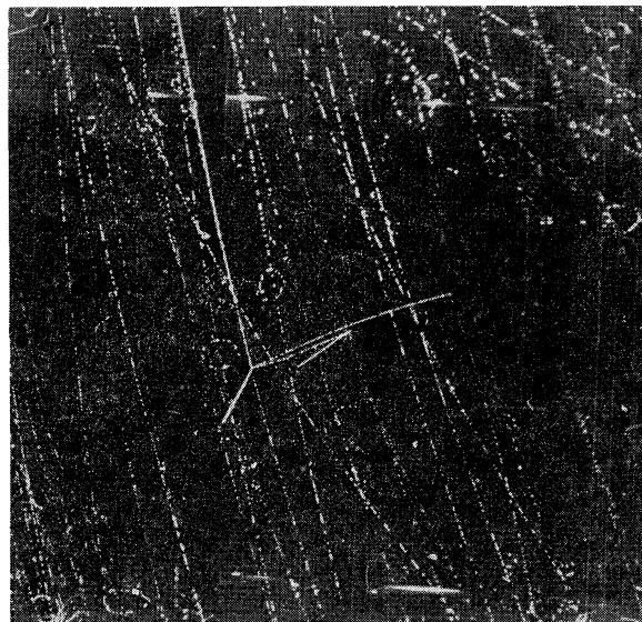
FIG. 15. An antiproton enters at top left of picture and makes a heavy track until it annihilates near center of picture. The longer of the two prongs on the right may be seen to decay, sending a minimum-ionizing particle down and out of the bottom of the picture. This is a K^+ \rightarrow \pi^+ + \pi^0 at rest. Event number 36046.
