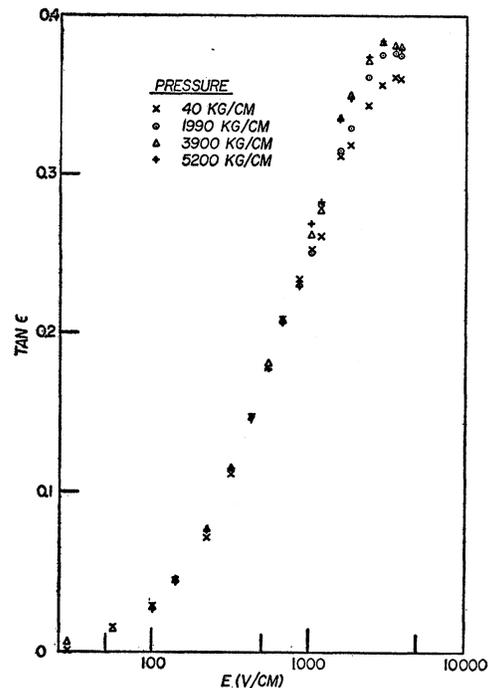
FIG. 4. The variation with pressure of  $\tan \epsilon$ , the tangent of the angle between the electric field and the current, measured at 77°K for a sample the orientation of which was chosen to give maximum effect.
