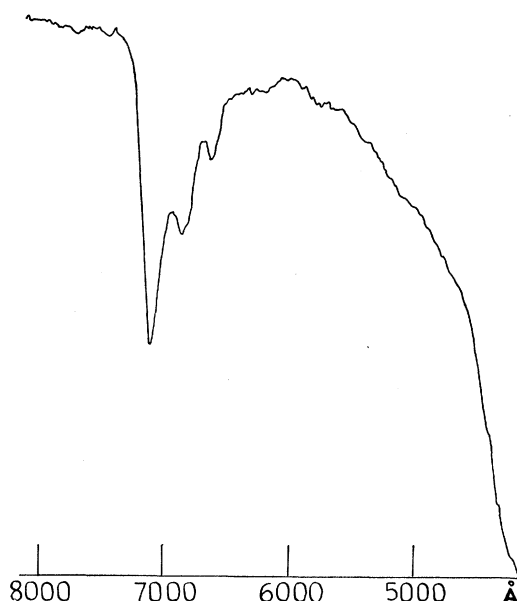
FIG. 6. The optical spectrum of ZnS in the visible range.
