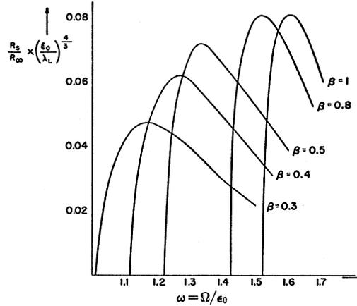
FIG. 1. The ratios of the surface resistance for a superconductor to the normal resistance in the extreme anomalous limit,  $R_s(\Omega)/R_\infty(\Omega)$ , as a function of frequency, calculated for various values of  $\beta = (1 - \sigma')/\sigma' N(0) V$ , where  $\sigma'$  is the parameter of the angular dependence of  $V(k, k')$ .
