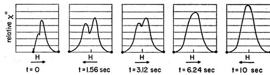
FIG. 2. A sequence of tracings made from a single photograph showing the recovery of the saturated portion of the resonance absorption at 4°K. The high-frequency field was  $4.4 \times 10^{-4}$  gauss. The sweep is 156 gauss between extremes and the center of the trace is near 3200 gauss. The concentration of  $F$  center was  $4.8 \times 10^{17}$  cm<sup>-3</sup>.
