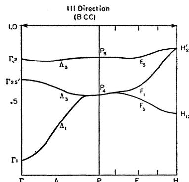
FIG. 2. Plot of energy bands  $E_n(k)$  for bcc iron obtained via APW method (reference 3) using potential of reference 8. Energy in Rydbergs. Labeling that of Bouckaert, Smoluchowski, and Wigner.<sup>9</sup>
