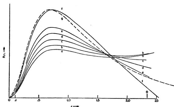
FIG. 3. Plot of radial wave functions  $P_2(r)$  [see Eq. (3)] for  $d$  band energies. Functions are *not* normalized. (a)  $E = E(H_{12}) = 0.41$  Rydberg (bottom of  $d$  band); (b)  $E = 0.45$  Rydberg; (c)  $E = 0.55$  Rydberg; (d)  $E = 0.65$  Rydberg; (e)  $E = 0.75$  Rydberg; (f)  $E = E(N_2) = 0.88$  Rydberg (top of  $d$  band); and (g) atomic  $3d$  function [J. H. Wood and G. W. Pratt, Jr., *Phys. Rev.* **107**, 995 (1957)].
