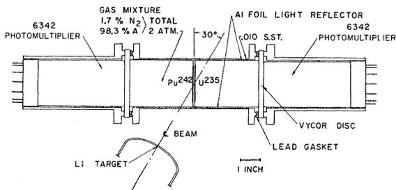
FIG. 1. Back to back gas scintillation counter.
