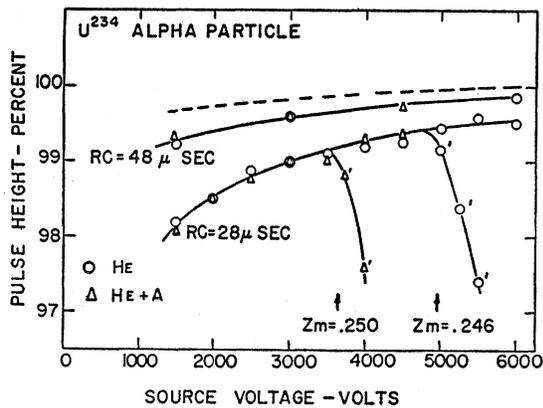
Fig. 3. Helium and helium plus argon saturation curves.
