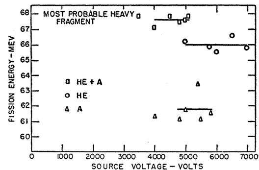
FIG. 6. Heavy fragment saturation curves, method II.
