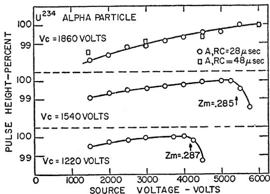
Fig. 4. Argon alpha saturation curves.
