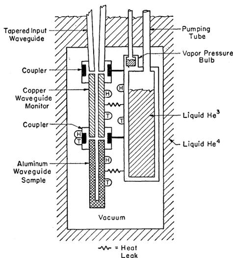
FIG. 3. Schematic diagram of the low-temperature part of the apparatus. The symbols  $H$  and  $T$  refer to heaters and carbon resistance thermometers, respectively. (See the text for the description of the functions of the various components.)
