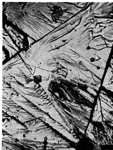
FIG. 3. Photomicrograph of a cleaved iron surface showing an area 0.0037 \times 0.005 square inch.
