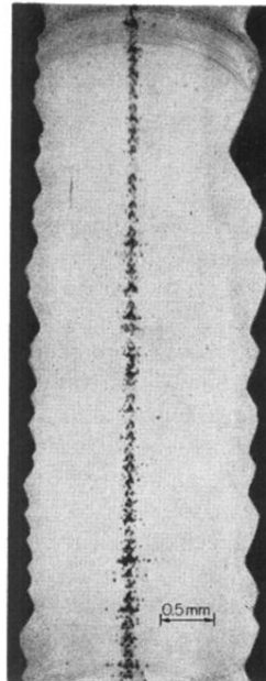
FIG. 7. Dendrite surface, etched.
