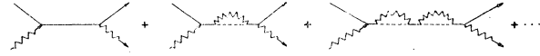
FIG. 3. Diagrams summed over in calculating phonon-polaron scattering with quasi-phonon (wavy lines) corrections. Solid lines represent the two-particle oscillator propagating in its ground internal state, and the dotted lines represent propagation in an arbitrary internal state.
