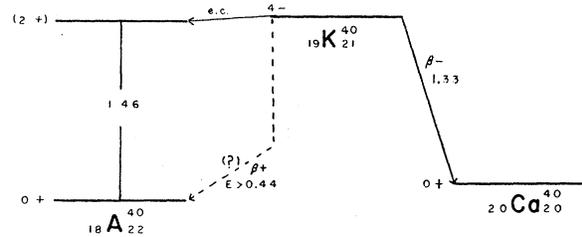
FIG. 3. Decay scheme of  $K^{40}$ .
