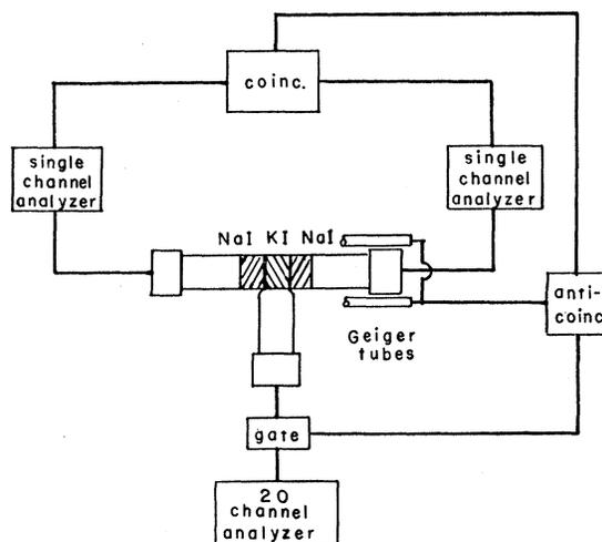
FIG. 1. Block diagram of triple coincidence system.
