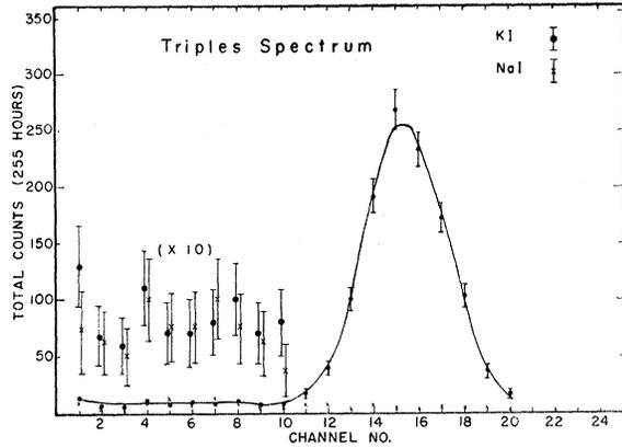
FIG. 2. Spectrum of triple-coincidence pulses from KI and NaI. The peak centered at channel 15 is due to pair production by the 1.46-Mev gamma ray.
