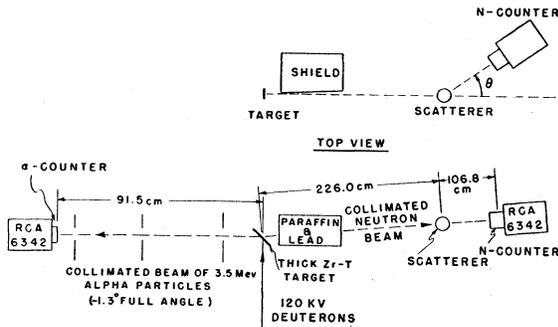
FIG. 1. Experimental arrangement for elastic scattering of 14-Mev neutrons.
