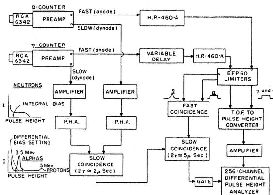
FIG. 2. Electronic circuitry. The limited and shaped alpha-particle pulses are 80  $\mu$ sec in duration and 5 volts in amplitude. The limited and shaped neutron pulses going to the time-of-flight-to-pulse-height converter have a duration of 80  $\mu$ sec and an amplitude of 5 volts and those going to the fast coincidence circuit have a duration of about 8  $\mu$ sec and an amplitude of about 2 volts.
