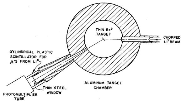
FIG. 1. Apparatus for measuring the angular distribution of short-lived radioactive products.
