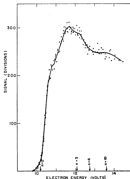
FIG. 6. Typical single observations of signal at low energies for both H and D. The results of each run are normalized to give the same area under the curve representing the excitation function.
