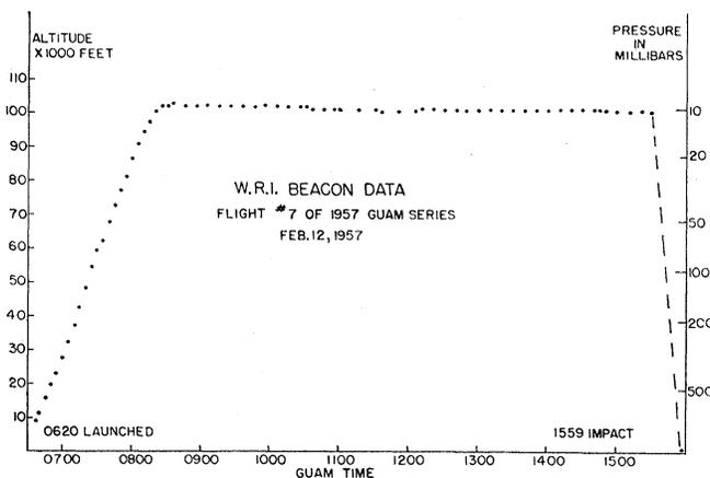
FIG. 1. Flight curve of stack.
